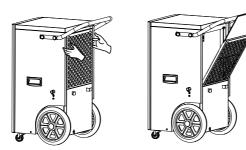
• To remove the air filter: Grasp the filter tab and pull it obliquely up to take out the entire filter, as illustrated below.
