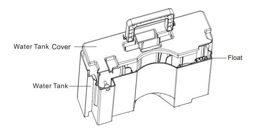
Tips: After proper tank installation, allow 1-3 minutes for the water full light to reset. If the light persists: Unplug and reinstall the tank. Ensure the tank is clean and the machine is level. Contact our support if still unresolved.
